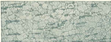
Fig. 6. Wire after many drawings loses much of its ductility, but when annealed at suitable high temperature, strain-distorted crystals rearrange themselves as shown.
