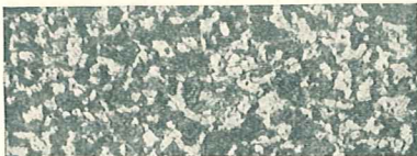
Fig. 2. Properly annealed sample of .45 per cent carbon steel, which has been restored from the condition referred to in Fig. 8.
