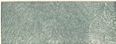
Fig. 7. Conditions of ordinary annealed steel containing 90-100 per cent carbon. Steel comparatively soft, of low strength and high ductility.
