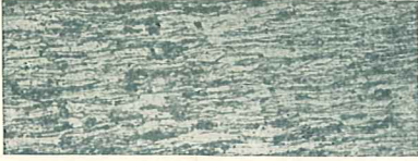
Fig. 5. Same wire after a number of drawings, with extreme elongation of crystals and obliteration of original boundary lines.
