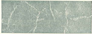
Fig. 8. Crystals of a steel containing .45 per cent carbon made coarse by overheating.
