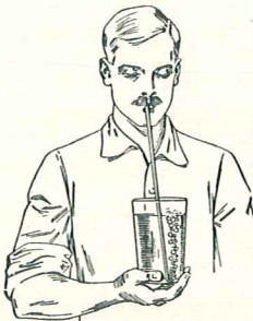
Bessemer process—blowing air up through vessel from bottom.
