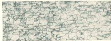
Fig. 4. Same wire drawn once through the die—crystals elongated in direction of drawing, but keeping original area.
